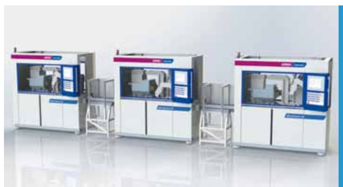
Example of special process: Three-component micro injection moulding machinery (courtesy of FOTEC Forschungs- und Technologietransfer GmbH and Wittmann Battenfeld GmbH).
